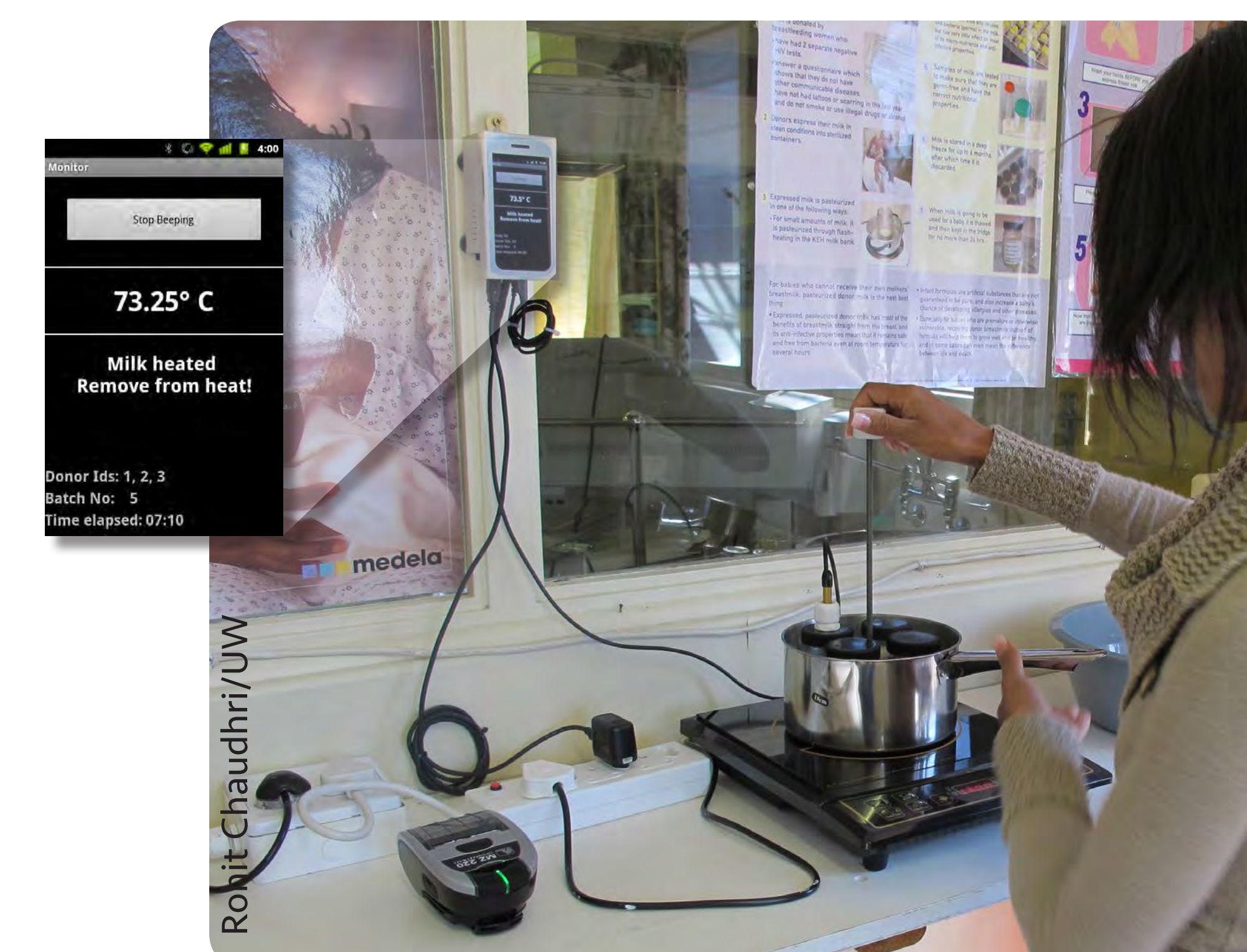
FoneAstra milk pasteurization monitor being used to treat donor milk at neonatal intensive care unit in South Africa.
