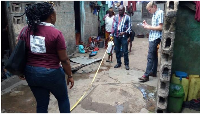
PATH and Population Services International project team members take measurements to determine space constraints for septic tanks in the compounds and households. Photo: Population Services International.
