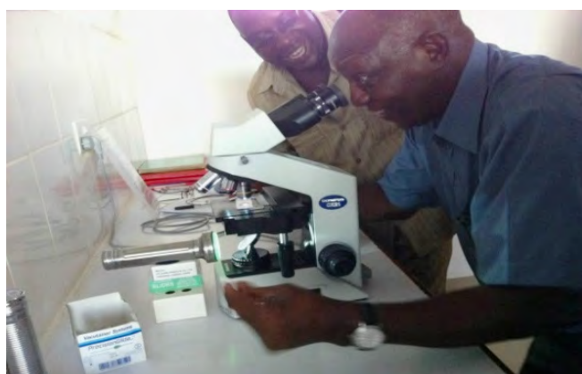
A PATH laboratory technical officer uses a torch as a light source in a microscope to perform a sputum examination.
