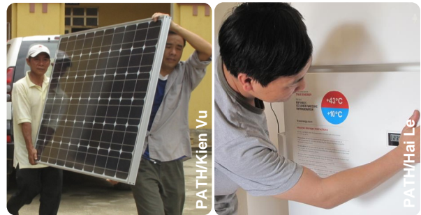
A small solar array can power this direct-drive refrigerator.
