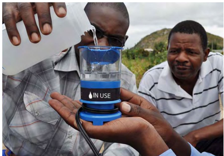
The field trials in Zimbabwe identified unanticipated challenges to using the SE200, such as difficulty filling the device to a consistent volume when no flat surfaces were available.
